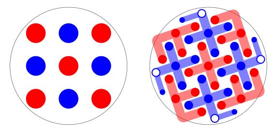
The white circles mark where splits are used, showing the diameter of the connection to the next layer. Note that the only locations which are adjacent to only two dots of the other color are the split blue tubes. This can act as a guide to where splits are needed, but ultimately it is about improving paths on the next level.
