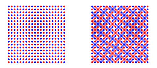
The centers of the connected tubes also form a regular grid, although rotated by about  $-26.6^{\circ}$  (tan<sup>-1</sup> - 1/2). Also, since five tubes are feeding into one, we assume the diameter of the tubes will increase by  $\sqrt{5}$ , as does the grid spacing. Again, one can connect the tubes together using the same (but rotated) pattern.
